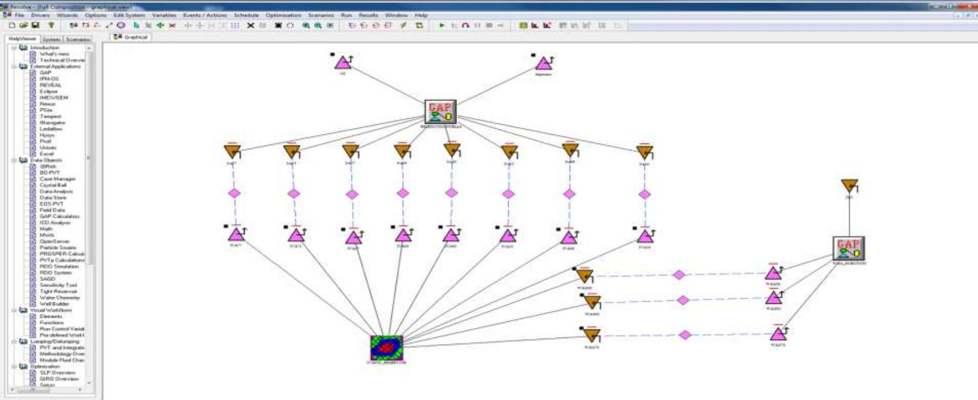
*EOR Ivanić- Existing Reservoir model is not combined with surface GAP model and without bottlenecks. With integration of these models it is possible to predict bottlenecks in surface equipment to act proactive and to remove them to achieve maximum production potential from reservoir.*
