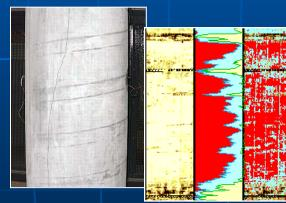
Micro annulus; Cement cracks
