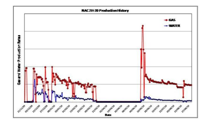
"[W]e observe that after extended shut-in the rate increases with a higher decline, the pressure is recharged but shows higher decline. . ."
