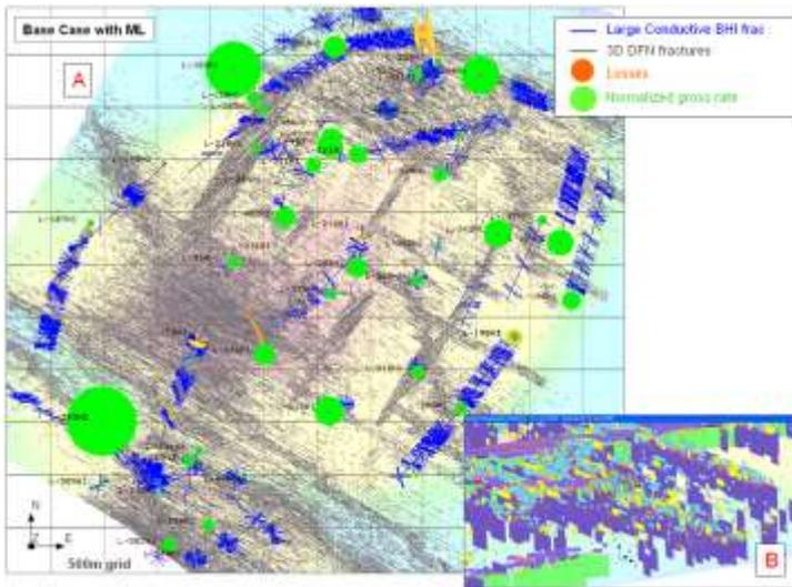
DFN model based on wellbore image data + seismic and fitted to a fracture corridor concept (from PhD work by Salah al Dhahab)
