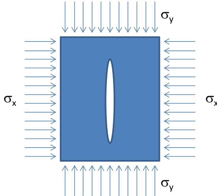
Note: this is the model used to calculate wellbore stability, and it is wrong
