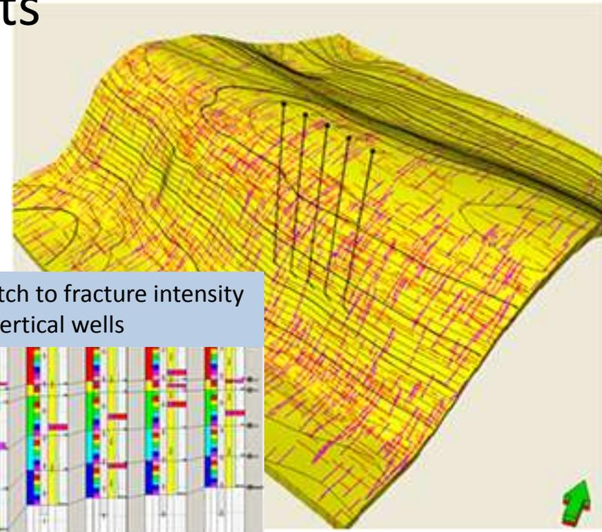
Sector model of a fractured carbonate reservoir with 12 fracture corridors (after Questiaux et al 2010)
