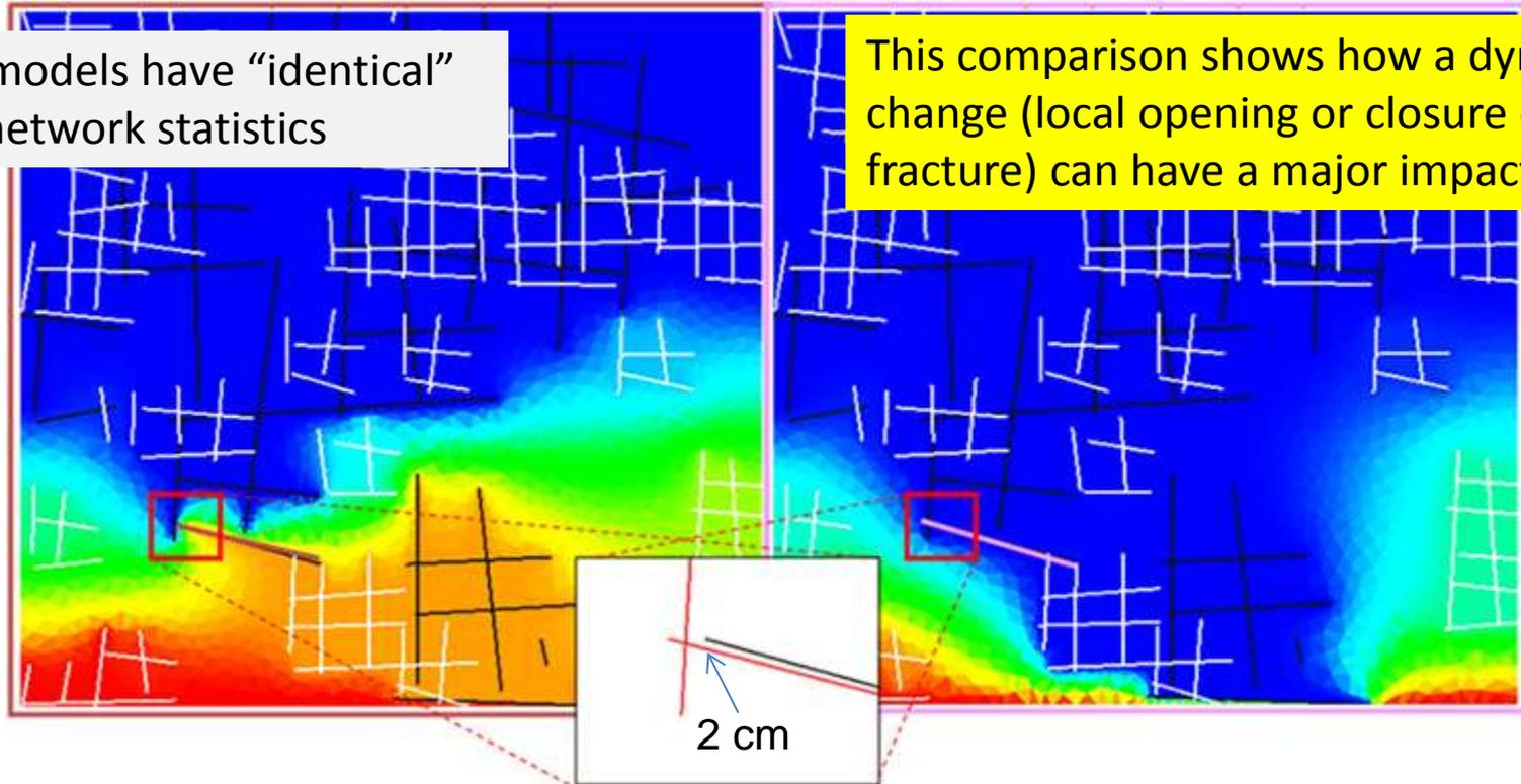
Colours show pressures. Black and white lines are fracture traces. Difference between models is very small – only a tiny change in connectivity of the fracture network (see inset box). The effective perm of the right model is **6X** that of the left one. This change cannot be predicted from fracture population statistics.
