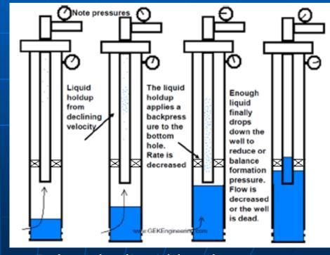
Below the liquid level <del>></del> greater pressure increment
