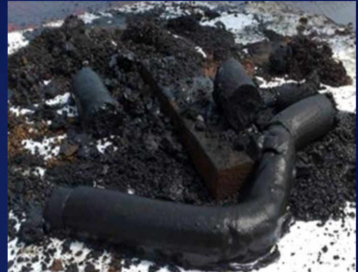
Corrosion Byproducts: Oily Iron Sulphide and Iron Oxide in an Injector
