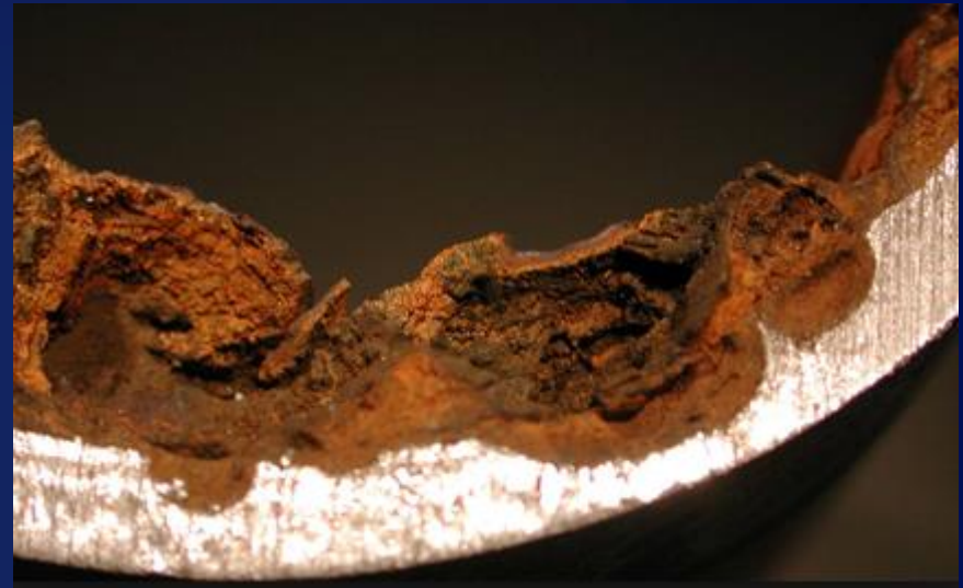
Pipeline Under Deposit Corrosion
