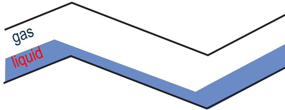
$$\left[ \frac{\Delta p}{\Delta L} \right]_{\text{Total}} = \underbrace{\left[ \frac{\Delta p}{\Delta L} \right]_z}_{\text{elevation}} + \underbrace{\left[ \frac{\Delta p}{\Delta L} \right]_f}_{\text{friction}} + \underbrace{\left[ \frac{\Delta p}{\Delta L} \right]_a}_{\text{acceleration}}$$
