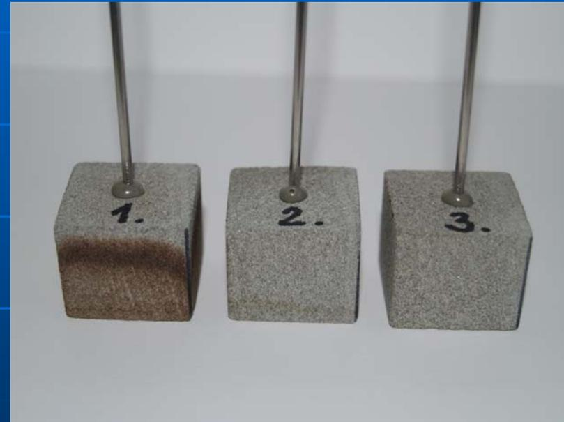
Semiautomatic apparatus for imbibition tests
