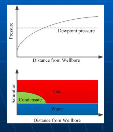
Total Skin:  $s_t = s + s_{2p}$ Skin effect caused by condensate drop-out:  $s_{2p} = \frac{2.3025}{|m|} \int_{p}^{p_{dew}} \left[ \frac{k_{rg}(S_{wi})}{\mu_{g} \cdot Z_{g}} - \left( \frac{k_{ro}}{\mu_{g} \cdot Z_{g}} + \frac{k_{rg}}{\mu_{g} \cdot Z_{g}} \right) \right] dp$
